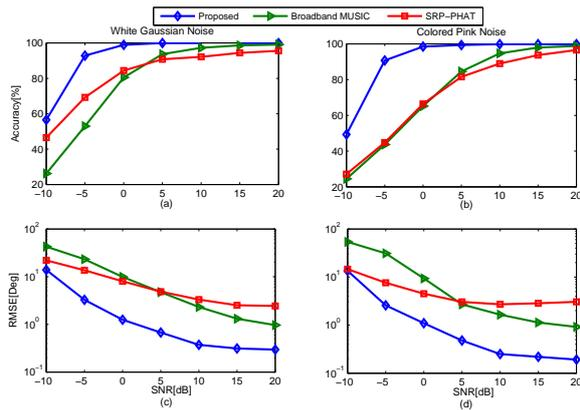
Figure 2: Estimation performance of different algorithms. (a)(c) Accuracy and RMSE with white Gaussian noise. (b)(d) Accuracy and RMSE with colored pink noise. The error tolerance for Accuracy is  $5^\circ$
