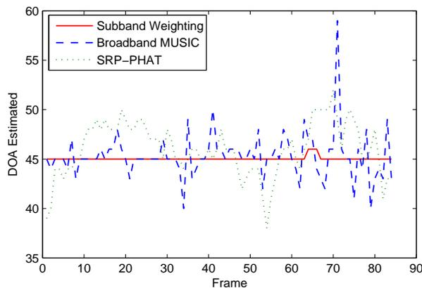
Figure 3: DOA estimates for a continuous speech with 8dB SNR white Gaussian noise. The true DOA is  $45^\circ$ .
